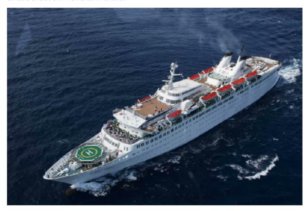
TWIN SCREW CLASSIC CRUISE VESSEL DIMENSIONS LOA 160.13M X BEAM 22.823M X 6.72 METERS DRAFT GRT 15,781
